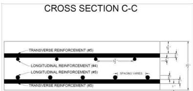
Figure 3.35. Bridge A1297 Deck Cross Sections
