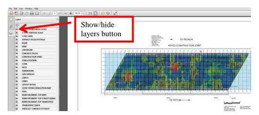
Figure F.1. Layers in Digital Drawing
