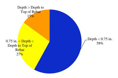
Figure 3.32. Bridge A1479 Lidar Depth of Concrete Removal Results
