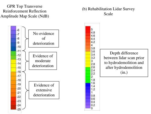
Figure C.1. Bridge A1297 GPR Map Scale (a) and Lidar Survey Scale (b)
