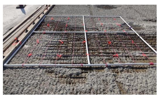
Figure 3.11. Grid Used to Obtain Manual Depth Measurements
