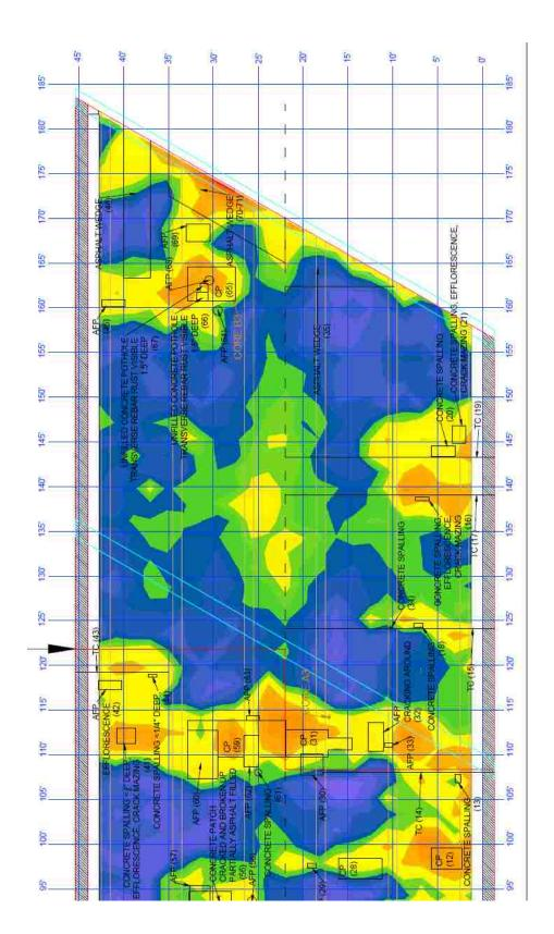
Figure C.7. Bridge A1297 Deck Investigation Drawing, GPR Results, Section 2 (95 ft. – 185 ft.) SPAN 3
