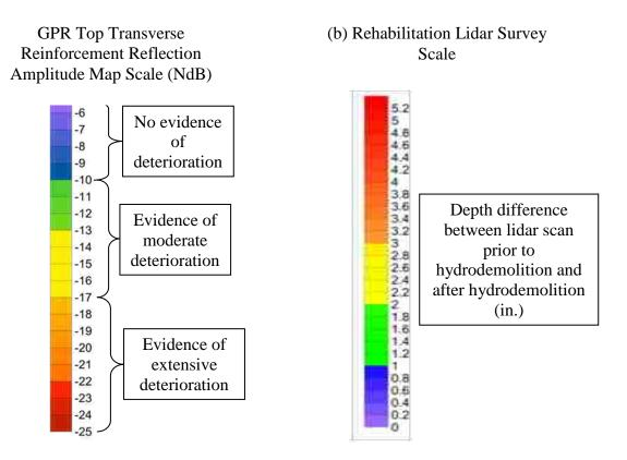
Figure A.1. Bridge A1479 GPR Map Scale (a) and Lidar Survey Scale (b)
