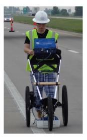
Figure 3.4. GSSI 1.5 GHz Ground Coupled GPR System
