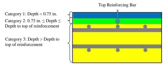
Figure 3.13. Categories of Material Depth Removal during Rehabilitation
