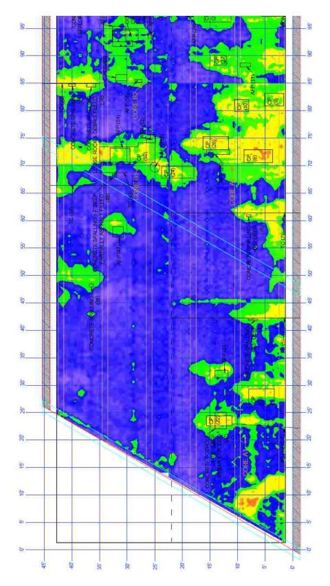
SPAN 1 SPAN 1 Figure C.5. Bridge A1297 Deck Investigation Drawing, Lidar Survey Results, Section 1 (0 ft. – 95 ft.)
