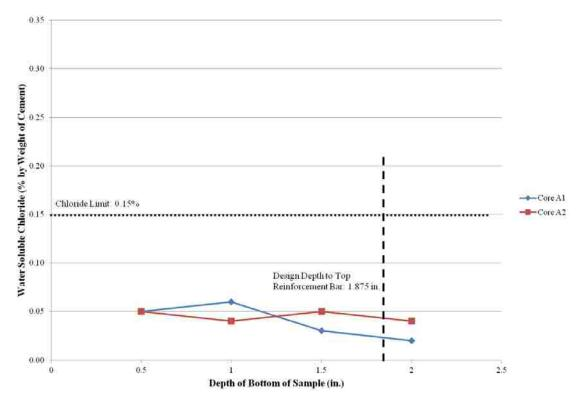
Figure 3.43. Bridge A1297 Chloride Ion Content Results
