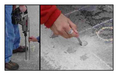
Figure 2.11. Pulverization Using a Rotary Hammer (Left) and Sample Extraction (Right) for Chloride Ion Determination
