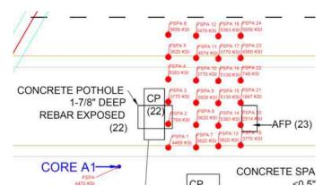
Figure 3.5. Sample PSPA Data Plotted on Bridge Deck Drawing
