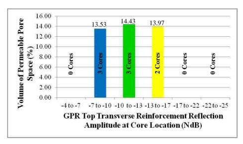
Figure 4.3. Volume of Permeable Pore Space Compared to GPR Amplitude for Bridge A1479
