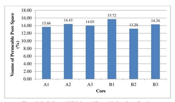
Figure 3.42. Bridge A1297 Volume of Permeable Pore Space Results
