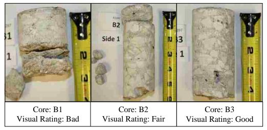
Figure D.1. Bridge A1297 Core Photographs
