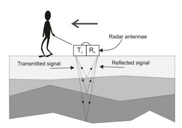
Figure 2.7. GPR Operating Principle [27]
