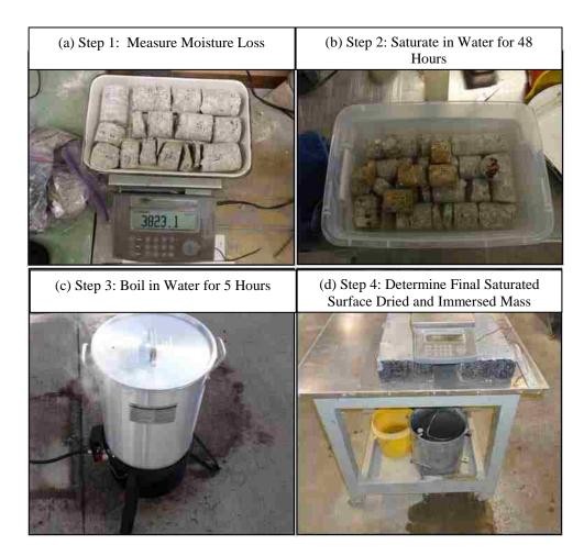
Figure 3.8. Process of Determining Volume of Permeable Pores
