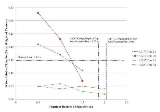
Figure 4.5. Bridges A1479 and A1297 Chloride Ion Concentration Results
