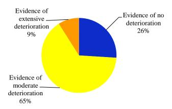
Figure 3.21. Bridge A1479 Deck Deterioration Levels Based on GPR
