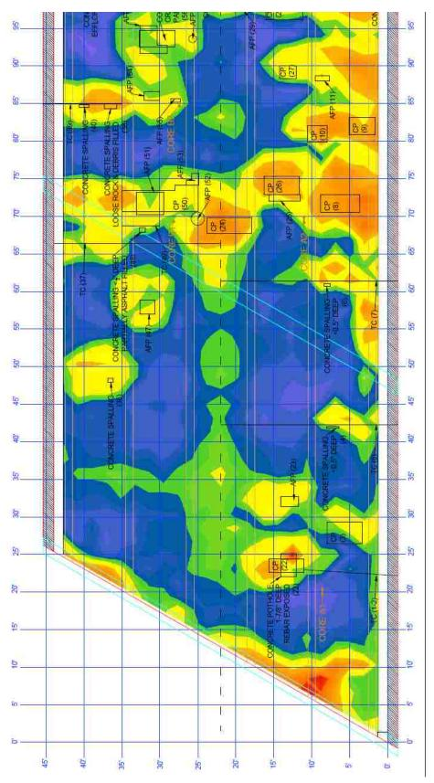
$_{\odot}$  SPAN  $_{\odot}$  Figure C.4. Bridge A1297 Deck Investigation Drawing, GPR Results, Section 1 (0 ft. – 95 ft.)
