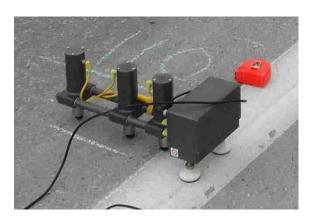
Figure 2.9. Portable Seismic Property Analyzer (PSPA)
