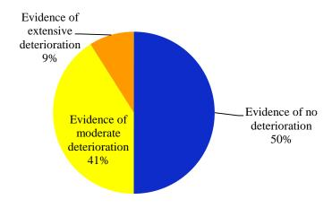
Figure 3.38. Bridge A1297 Deck Deterioration Levels Based on GPR
