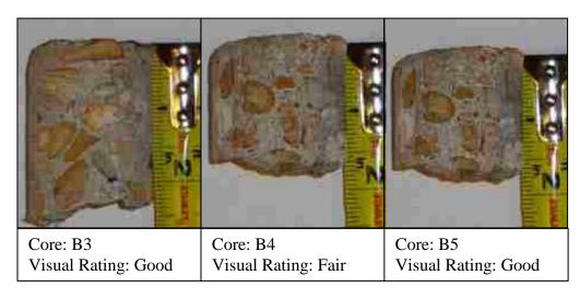
Figure 3.23. Bridge A1479 Cores and Visual Core Ratings
