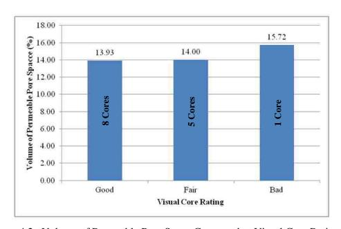
Figure 4.2. Volume of Permeable Pore Space Compared to Visual Core Rating for Bridges A1479 and A1297 Combined
