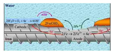
Figure 2.1. Steel Corrosion Mechanism [2]
