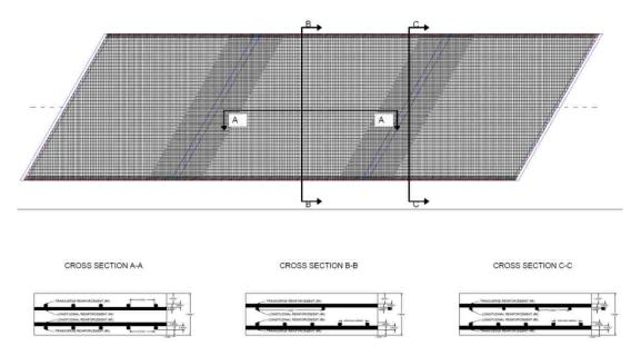
Figure 3.2. Sample Cross Section CAD Drawing of Bridge Deck
